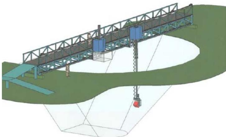
Figure 10: 3D model of the tronco-conical tank with rig showing one system under test at CTN.
