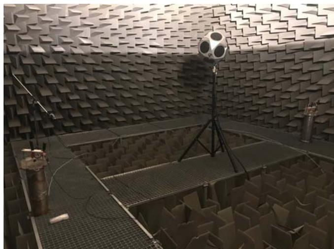
Figure 7: Practical layout for simultaneous calibration of 4 PAM devices in the QUIETMED project.
