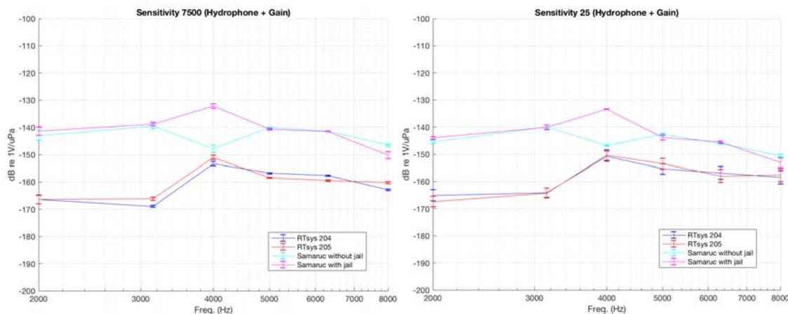
Figure 16: Sensitivity of 4 devices with a) 7500 cycles signals and b) with 25 cycles signals.
