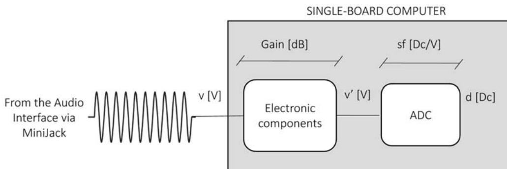
Figure 4: Block diagram related to the components within the Single-Board Computer.
