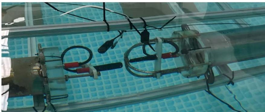
Figure 14: Detail of the placement of the 4 PAM devices to calibrate and the referenced one.
