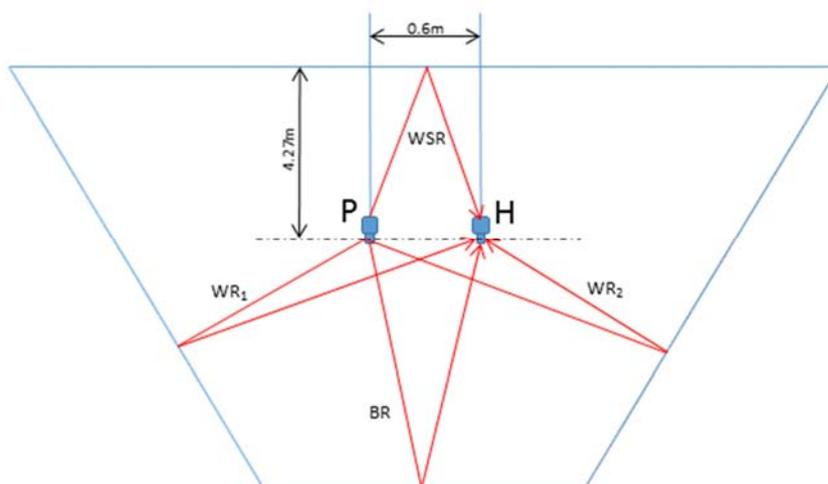
Figure 18. Scheme of direct path and early reflections from walls and water surface.
