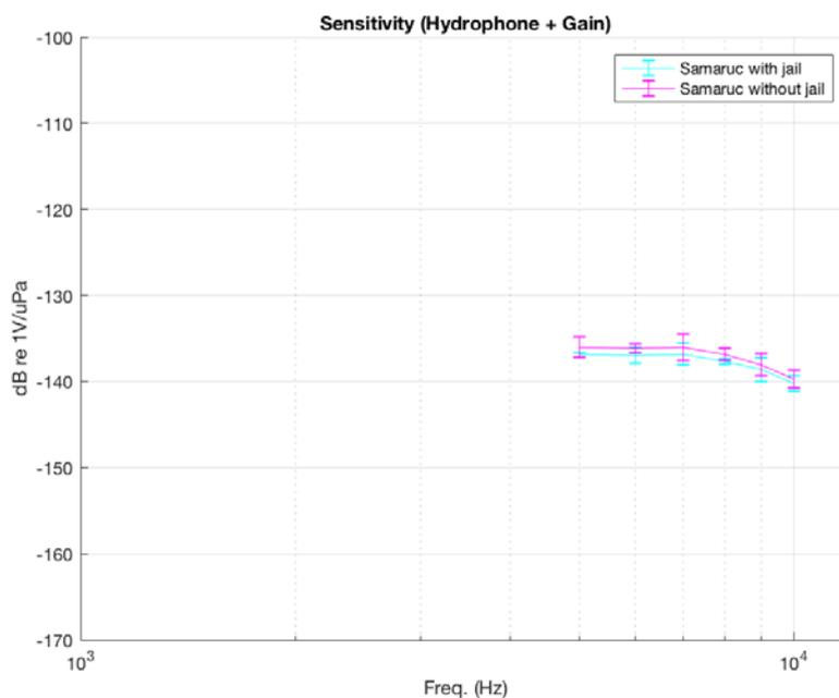
Figure 12: Sensitivity of SAMARUC PAM device with and without jail.
