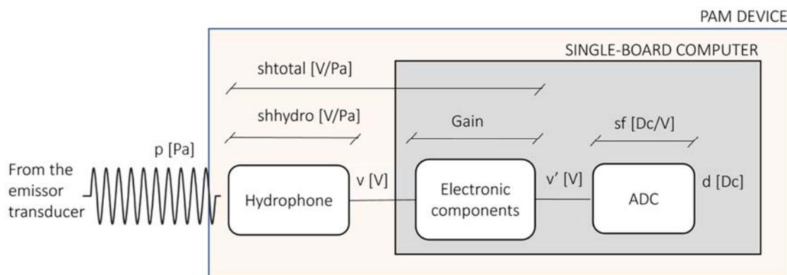
Figure 5: Block diagram related to a PAM device.
