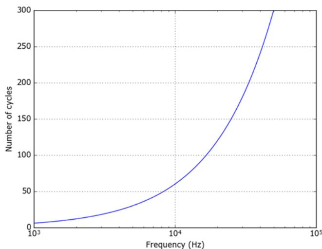
Figure 19. Number of cycles within the burst signal with 5.97 ms of echo-free time per frequency.
