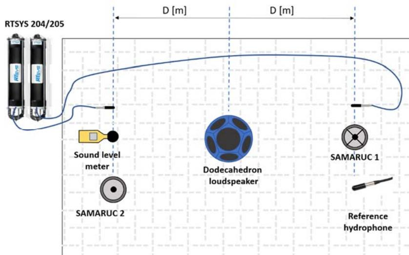
Figure 6: Layout of the elements for the calibration in the anechoic chamber.
