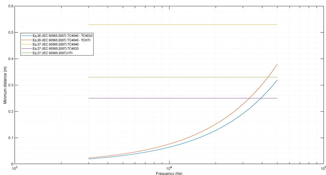
Figure 17. Minimum Distance from TC4040 to Reference hydrophones TC4033 and HTI-99.
