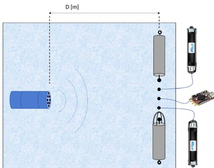
Figure 15: Layout for simultaneous calibration of 4 PAM devices in the QUIETMED project. Top view.
