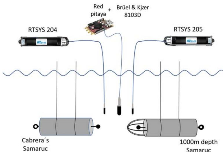
Figure 13: Layout for simultaneous calibration of 4 PAM devices in the QUIETMED project. View from the emitter transducer.
