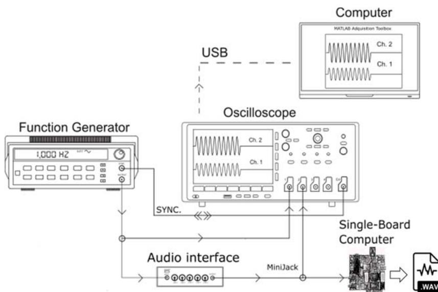
Figure 3. Layout of the set up in the calibration of the Single-Board Computer.
