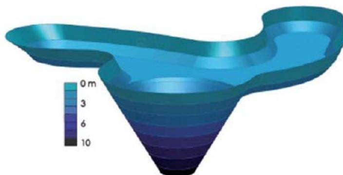
Figure 9: 3D model of the tronco-conical tank facility at CTN.
