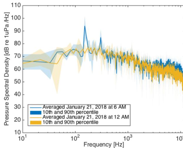
Figure 11: Acoustic noise spectral density for the averaged 21 January 2018 at 6 AM and at 12 AM. Statistical variance include as a shadow region the 10<sup>th</sup> and 90<sup>th</sup> percentiles as well as the mean in continuous line.
