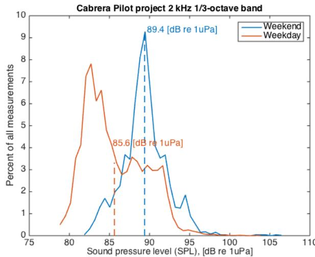
Figure 10: Level histograms for 2 kHz 1/3-octave band (Integration time T=30 seconds). Comparative for the overall weekdays and the overall weekends of the Cabrera Pilot Project.
