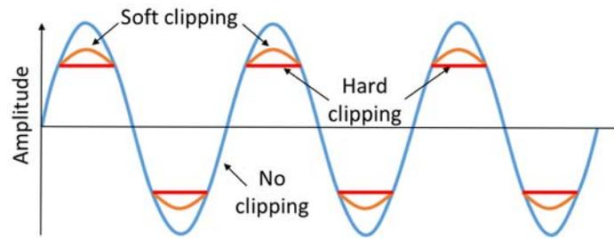
Figure 2: Hard clipping vs soft clipping.
