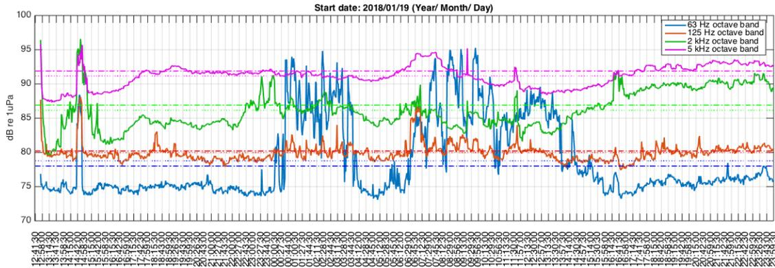
Figure 7: Ambient noise indicators vs time for the first two days of the Cabrera Pilot Project (Integration time T=30 seconds).
