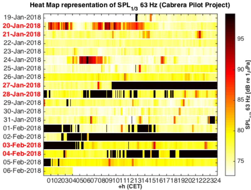
Figure 12: Example of a representation of the Cabrera Pilot project experiment ( $T_{bin}=15$  minutes and  $T=30$  seconds). The variable represented is the  $SPL_{1/3}$  in the central frequency of 63 Hz (weekends are shown in red).
