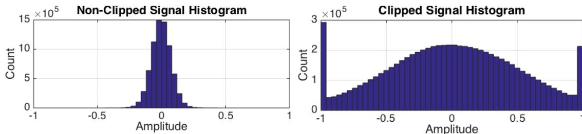
Figure 3: Left panel: histogram of a non clipped audio recording. Right panel: histogram of a heavily clipped audio recording.
