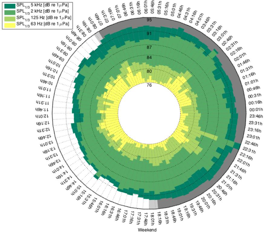
Figure 15: Polar area diagram of the Cabrera Pilot Project experiment. Ambient noise indicators averaged over the weekend. White/ grey sectors indicate day/ night calculated for longitude, latitude, and for all deployment dates using a generic astronomy calculator.
