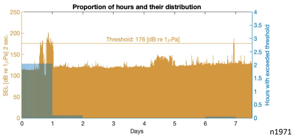
Figure 14: Time graph representation of the Sound Exposure Level and the proportion of time (hours in the day) above the given threshold. In the Figure TH=176 [dB re 1 μ Pa].
