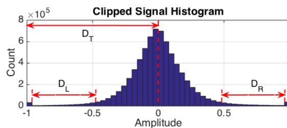
Figure 5: Measure clipping using histogram analysis.
