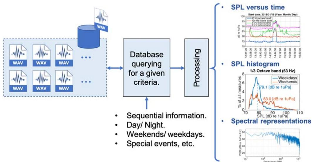
Figure 6: Different elements and stages involved in the creation of a graphical representation of ambient noise indicators.
