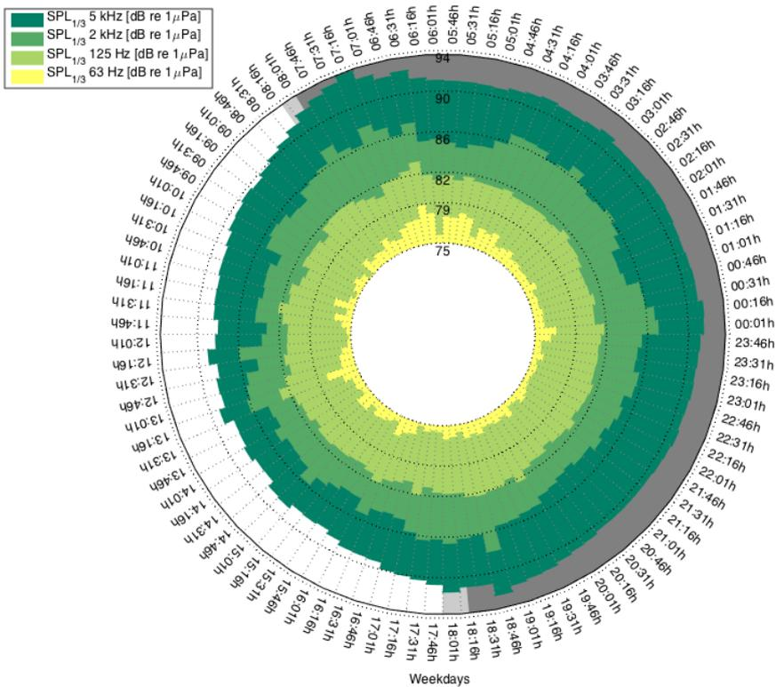
Figure 16: Polar area diagram of the Cabrera Pilot Project experiment. Ambient noise indicators averaged over the week days. White/ grey sectors indicate day/ night calculated for longitude, latitude, and for all deployment dates using a generic astronomy calculator
