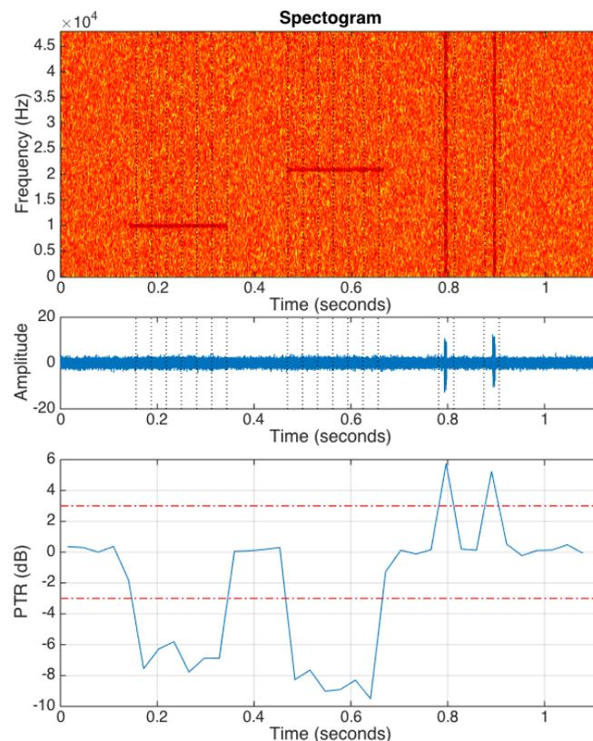
Figure 18: Top panel: spectrogram of an acoustic recording. Medium panel: temporal representation of the acoustic recording. Bottom panel: PTR of the acoustic recording.
