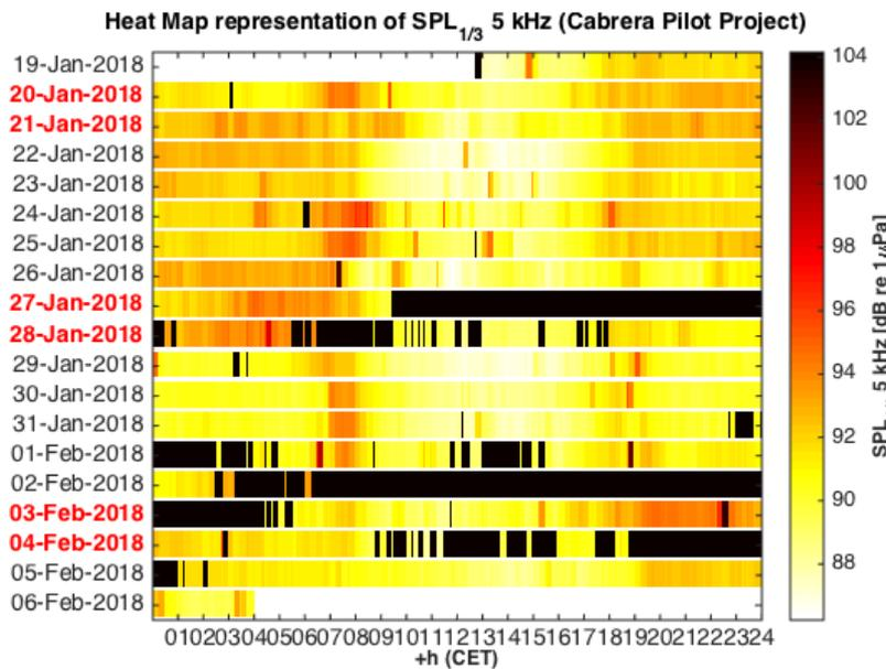
Figure 13: Example of a representation of the Cabrera Pilot project experiment ( $T_{bin}=15$  minutes and  $T=30$  seconds). The variable represented is the  $SPL_{1/3}$  in the central frequency of 5 kHz (weekends are shown in red). The figure allows to visualize the presence of vertical diel migrations of some fish species at sunrise/ sunset.
