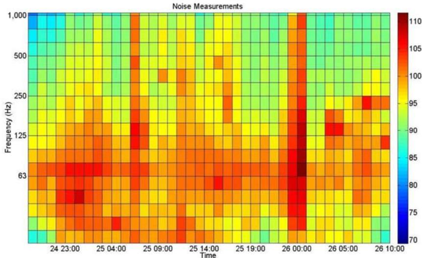
Figure 8: Octave noise levels calculated using data recorded by FORTH’s UL1 for south 1 (Greece south Pilot project).
