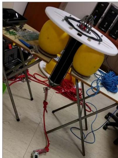
Figure 13: UM's circular rig attached with floaters (used in a test run)
