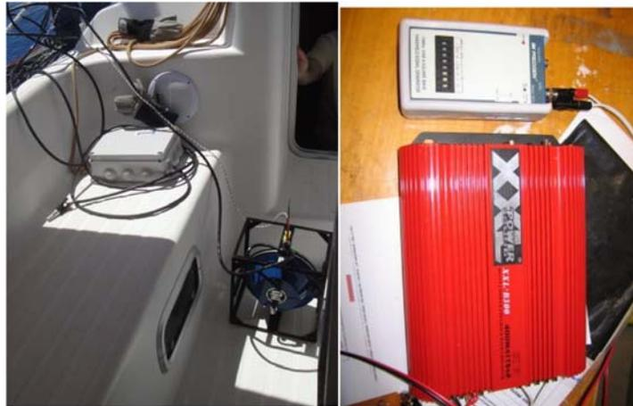
Figure 20: FORTH’s Lubell source prior to use (left) and the signal generator & amplifier (right)
