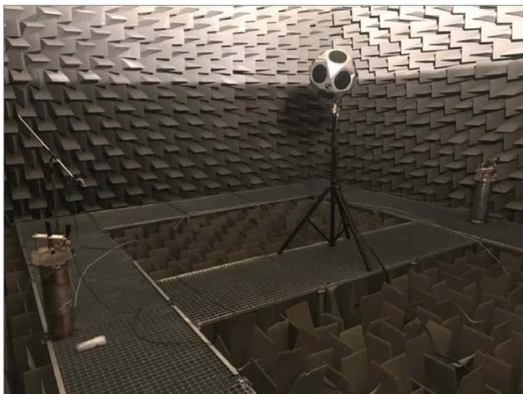
Figure 23: UPV's anechoic chamber layout for simultaneous calibration of 2 PAM devices
